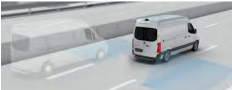
Blind Spot Assist with Rear Cross Traffic Alert can output visual and audible signals to help prevent accidents during lane changing, when reversing out of parking spaces and when exiting the vehicle.
