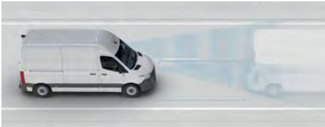
Active Brake Assist can help to avoid accidents with vehicle and crossing pedestrians ahead, or mitigate the effects of an accident.
