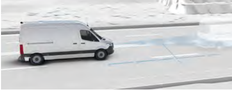
Active Distance Assist DISTRONIC can maintain the distance from the vehicle ahead as set by the driver and takes the strain off the driver in motorway driving or in stop-and-go traffic, for example.
