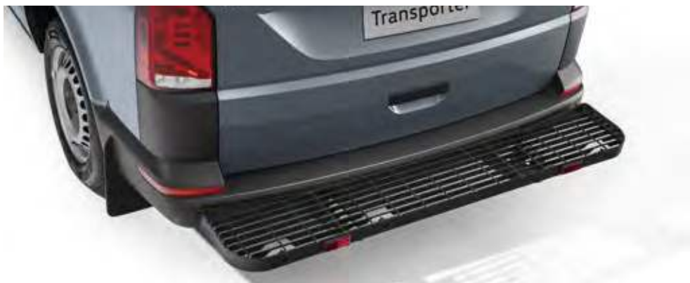
07 Rear technician step (to suit with and without towbar)
